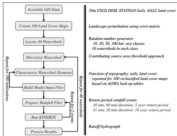
FIGURE 2. Flow Chart Illustrating the Procedures Used to Transform GIS Data Into Hydrologic Parameter Files for Input to KINEROS2.
