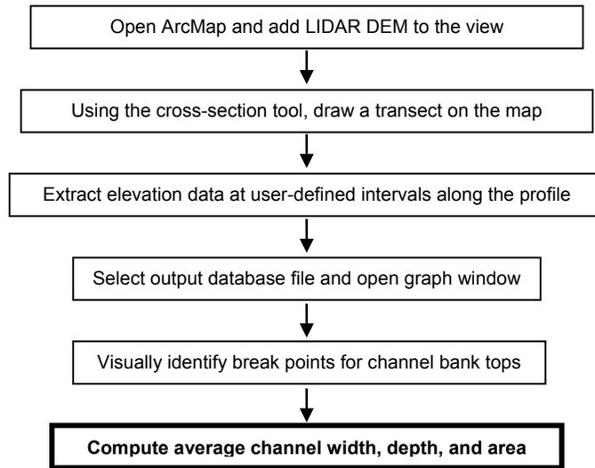
Figure 2. Diagram illustrating the methodology for extracting channel dimensions using the channel-characterization tool.
