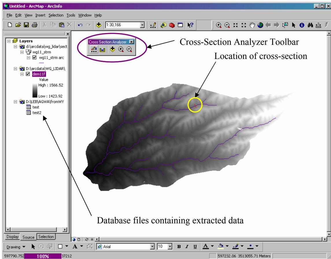
Figure 1. Screen capture showing the Cross-Section Analyzer toolbar, an example cross-section, and how the extracted data is made available to the graphing tool.
