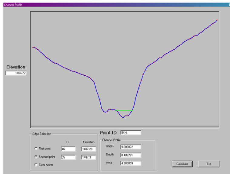
Figure 3. Screen capture of the graph window illustrating how channel banks are identified to permit channel width, depth, and area calculations. Units are inherited from the LIDAR data.
