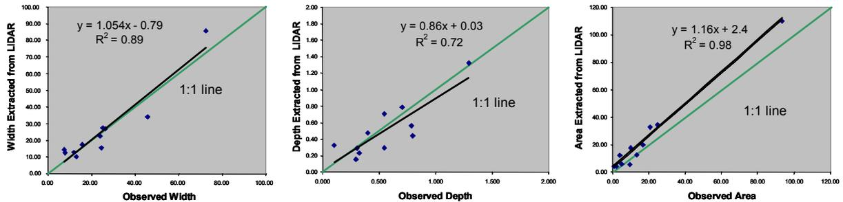
Figure 4. Estimated values for channel width (m), depth (m), and cross-section area (m<sup>2</sup>) extracted from LIDAR DEM plotted against values obtained from ground-based total station surveys. Linear regression models are shown on the figures with coefficients of determination.
