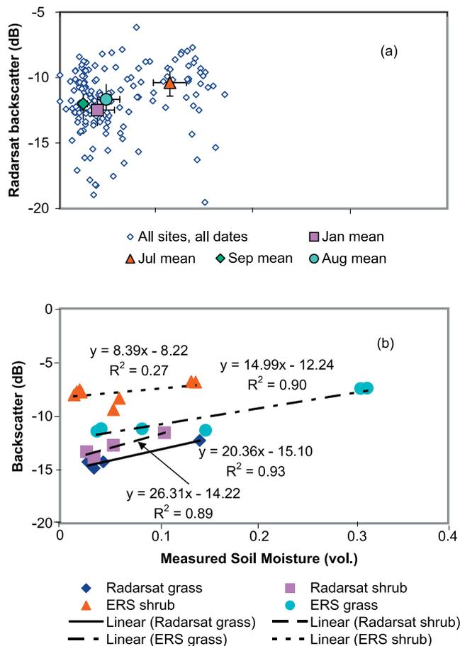
**Figure 3.** (a) Backscatter versus measured soil moisture by site and averaged for the watershed on four dates in 2003 using only RADARSAT observations. (b) Empirical relationships derived for homogenous areas of vegetation with both RADARSAT and ERS radar sensors across multiple dates.
