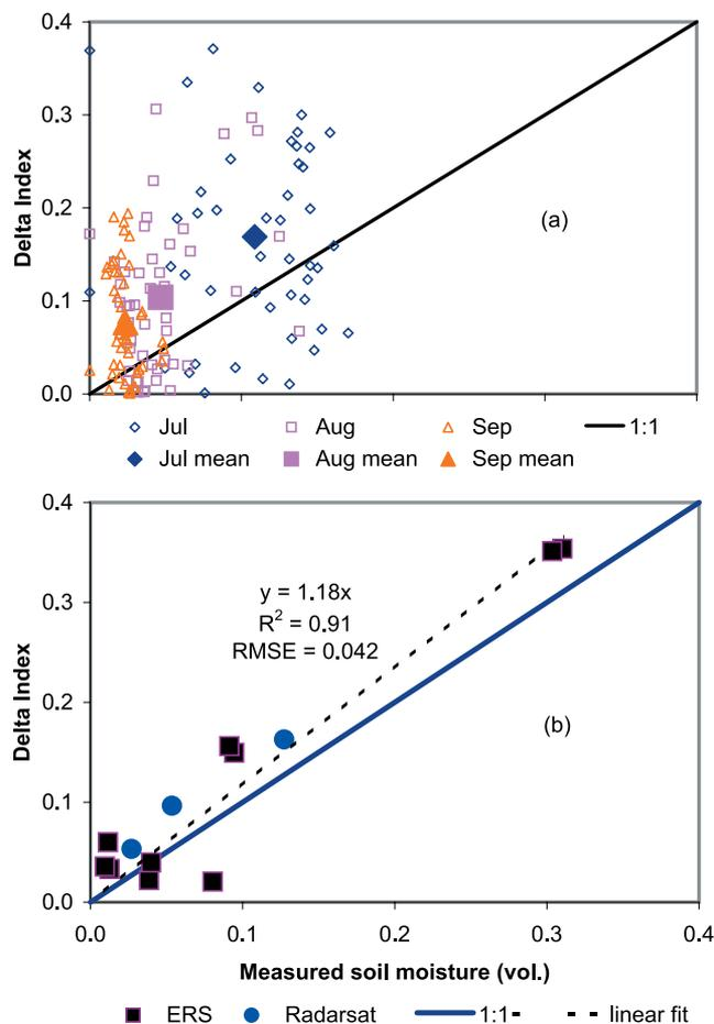
**Figure 6.** (a) Site-specific relationship between delta index and field measured soil moisture and averages of delta index and measured soil moisture. (b) Average delta index from 44 sites derived from RADARSAT imagery on three dates and delta index from three sites derived from ERS imagery on multiple dates versus soil moisture measured in the field. RMSE was computed as average difference between observed soil moisture and delta index.
