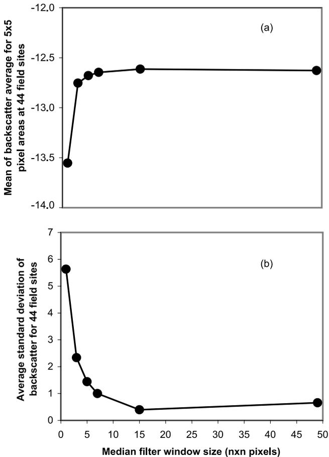
**Figure 2.** Effect of median filter window size on RADARSAT backscatter. (a) Mean backscatter from 44 field sites on three image dates in Walnut Gulch, Arizona. (b) Mean of standard deviations of backscatter from 44 field sites on three image dates. The area used to calculate standard deviation and mean for each of 44 sites was five by five pixels ( $91 \times 91$  m) nested over the  $35 \times 35$  m ground area sampled for soil moisture at time of satellite overpass.
