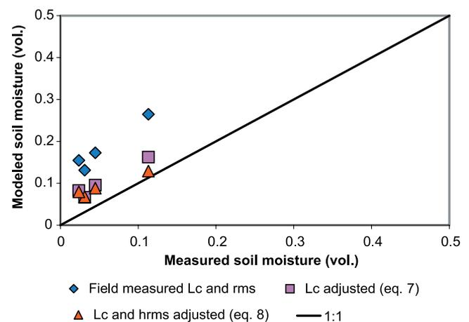
**Figure 5.** Modeled versus measured soil moisture for simulations at the watershed scale. The shift in data grouped by symbol represents  $L_c$  calibration suggested by Baghdadi et al. [2004] or  $L_c$  calibration plus  $h_{\text{rms}}$  adjustment. Only RADARSAT results are shown here because surface roughness data were not available for IEM simulation at the ERS-2 field sites.
