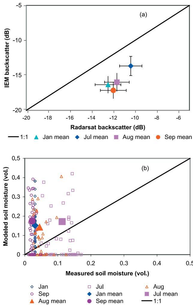
**Figure 4.** (a) Site-averaged IEM versus RADARSAT backscatter for 44 field sites sampled on four dates. The error bars represent backscatter standard deviation. (b) Site-specific modeled versus measured soil moisture and average modeled versus measured soil moisture. Only RADARSAT results are presented because surface roughness data were not available for IEM simulation at the ERS-2 field sites.
