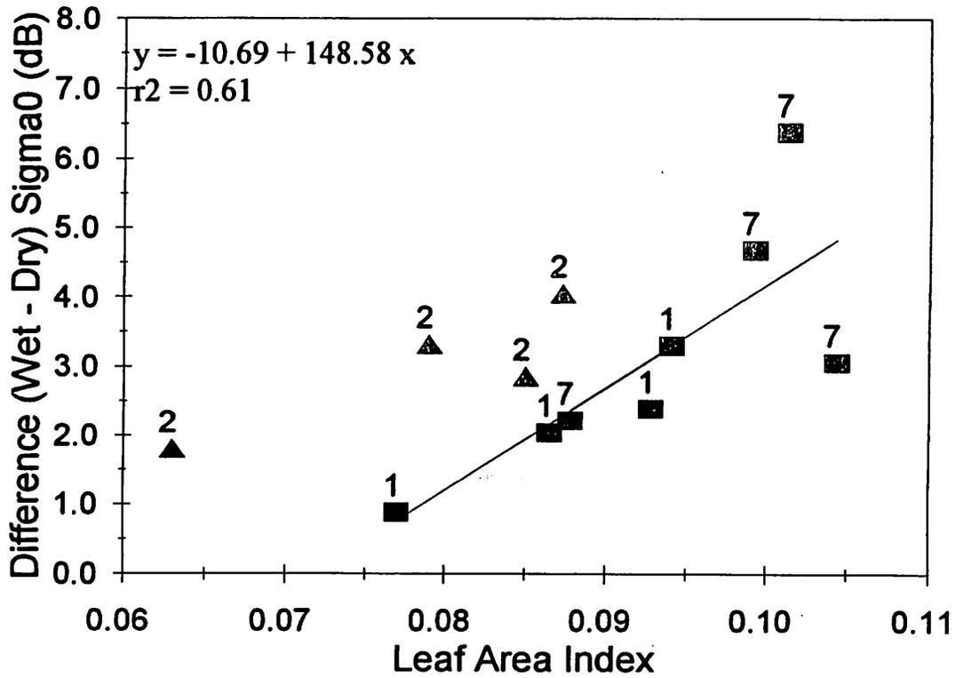
Fig. 3 – Scatterplot between radar backscattering coefficients and leaf area indices for MF stations 1, 2 and 7. Numbers above symbols represent MF sites. Data from MF 2 were not included in the regression analysis because of the probable high soil moisture content.
