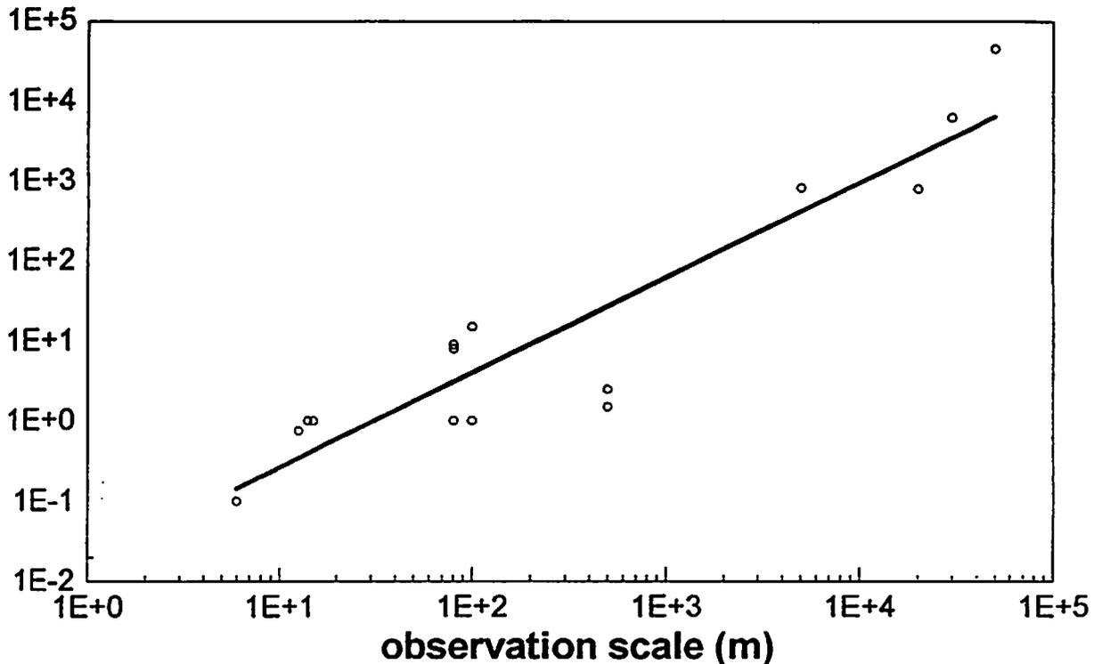
Fig. 1. Relationship between observation scale of the measurements and the calculated correlation scale for the Ks data of Table 1.
