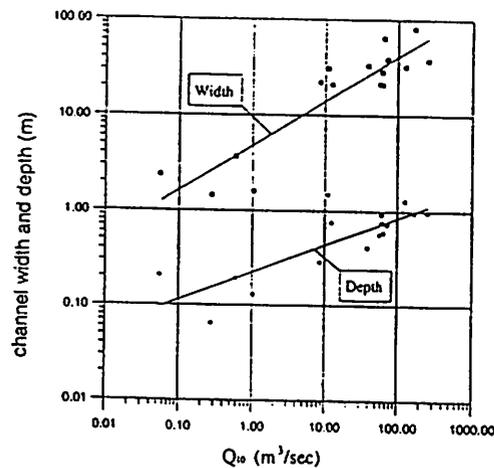
Figure 3: Hydraulic variables as a function of the 10-year peak flow
