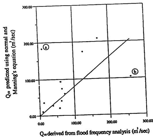
Figure 2: Comparison of  $Q_{10}$  values derived from flood frequency analysis and normal equation.
