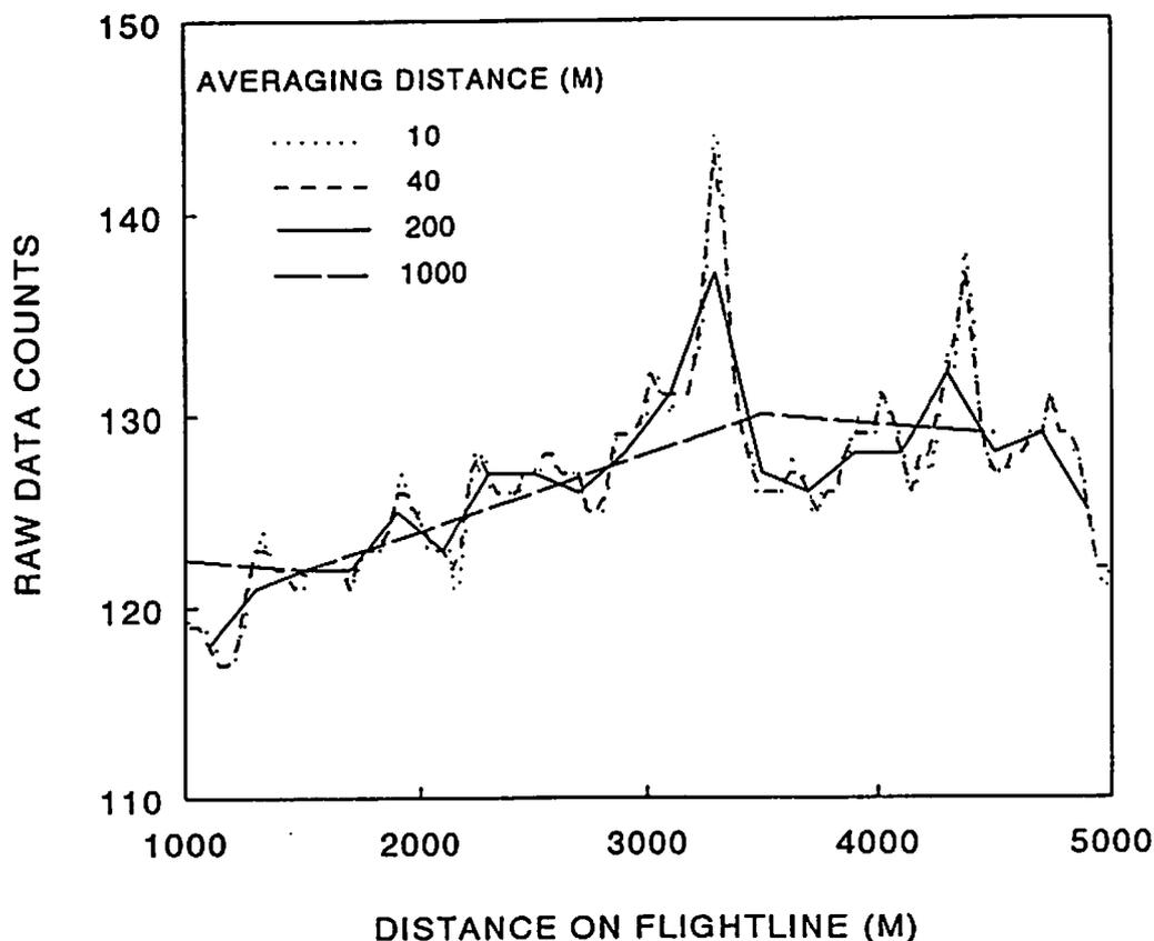
Figure 2. Effects of distance averaging on raw radiometer data, digital counts, patterns (a) X band and (b) L band.
