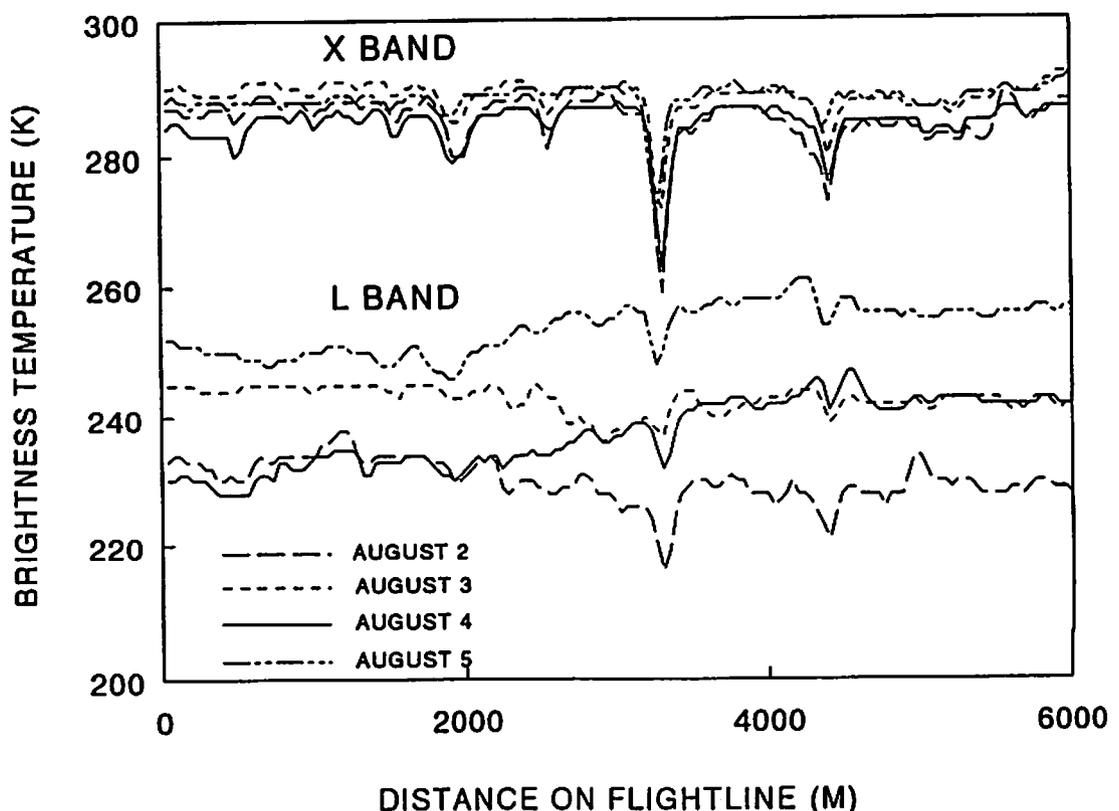
Figure 3. Microwave brightness temperature data collected on Walnut Gulch flightline 1 using (a) X band and (b) L band.
