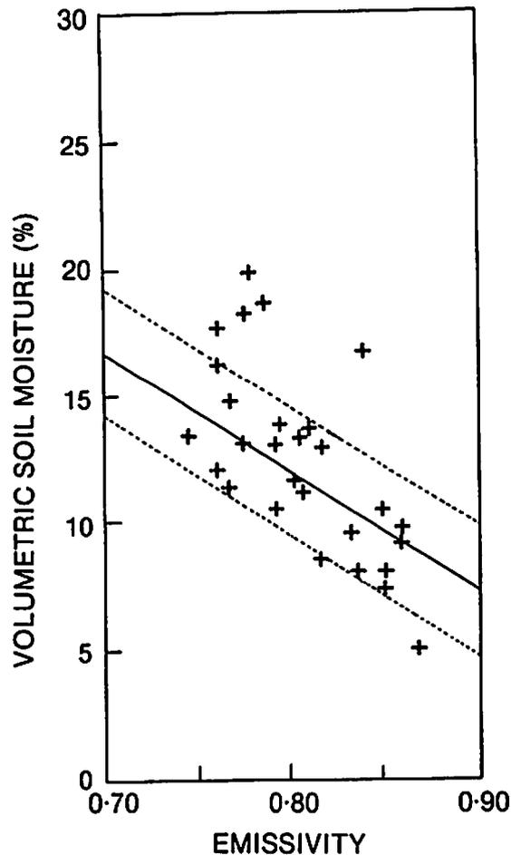
Figure 4. Soil moisture-emissivity relationship for the Walnut Gulch study site showing ground sampled and microwave estimated surface moisture. The solid line is the regression model and the dashed lines are the standard error.
