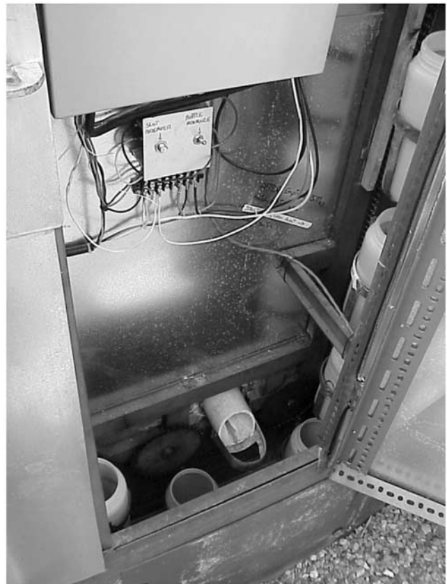
Figure 3. View of the inside of the instrument house at LH103 showing the sediment sample bottle carousel.
