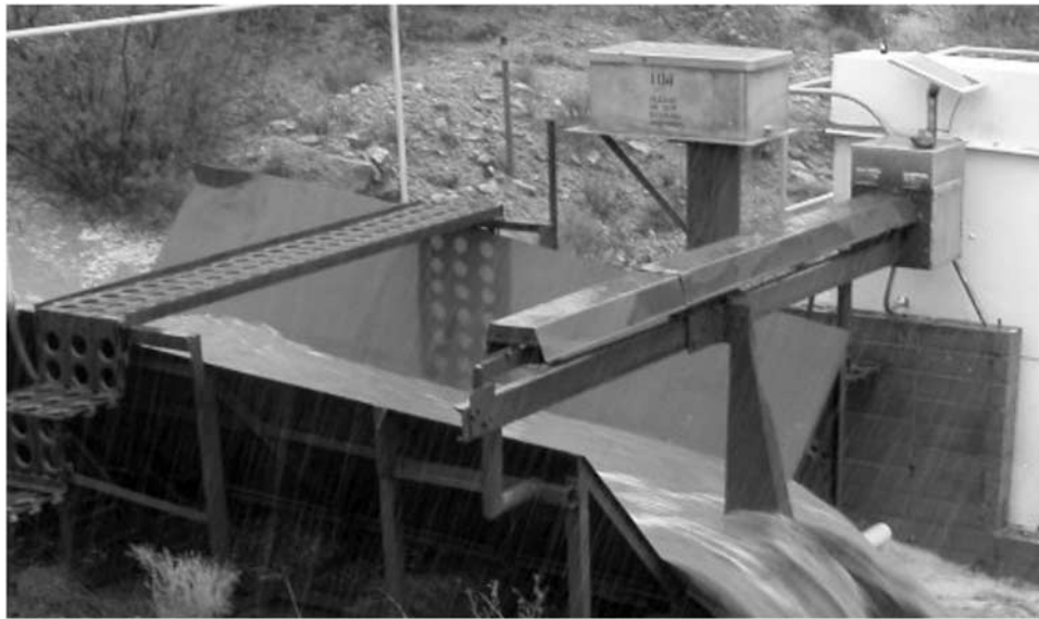
Figure 2. Smith-type supercritical flow flume and sediment sampler at LH104 showing traversing slot during a runoff event.
