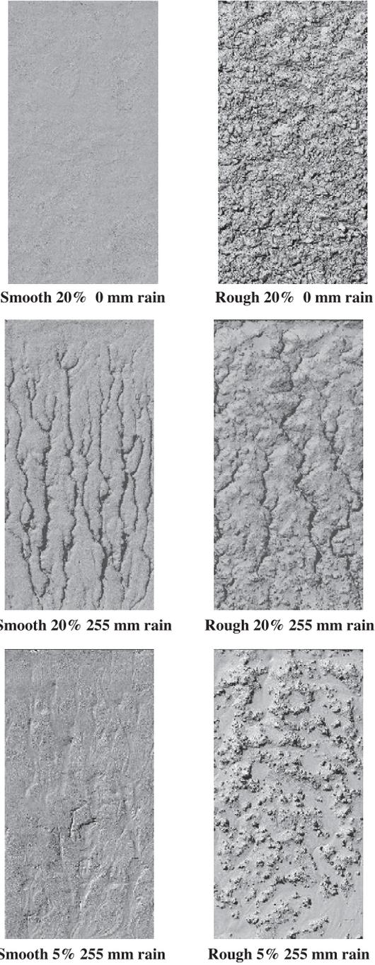
Fig. 1. Examples of the initial and final surfaces after 255 mm of rain. Plots were 2 m wide by 4 m long.
