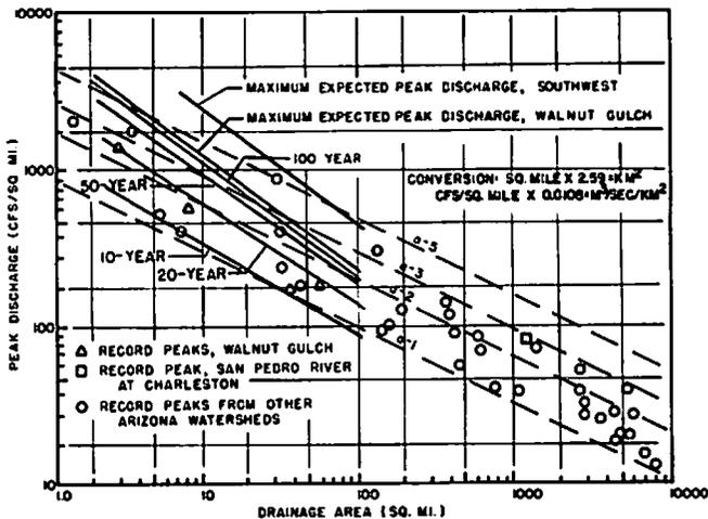
FIG. 7.—Comparison of Estimated Maximum Expected Peak Discharge and Estimated 10 yr, 20 yr, 50 yr, and 100 yr Peak Discharges for Walnut Gulch with Peak Discharges Versus Drainage Area for Arizona Flood Peaks
