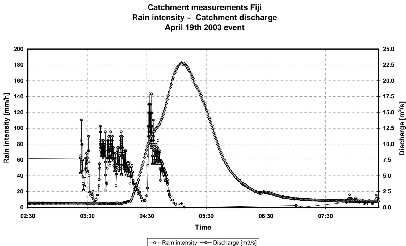
**Figure 1. Rain intensity and discharge from the catchment vs. time.**
