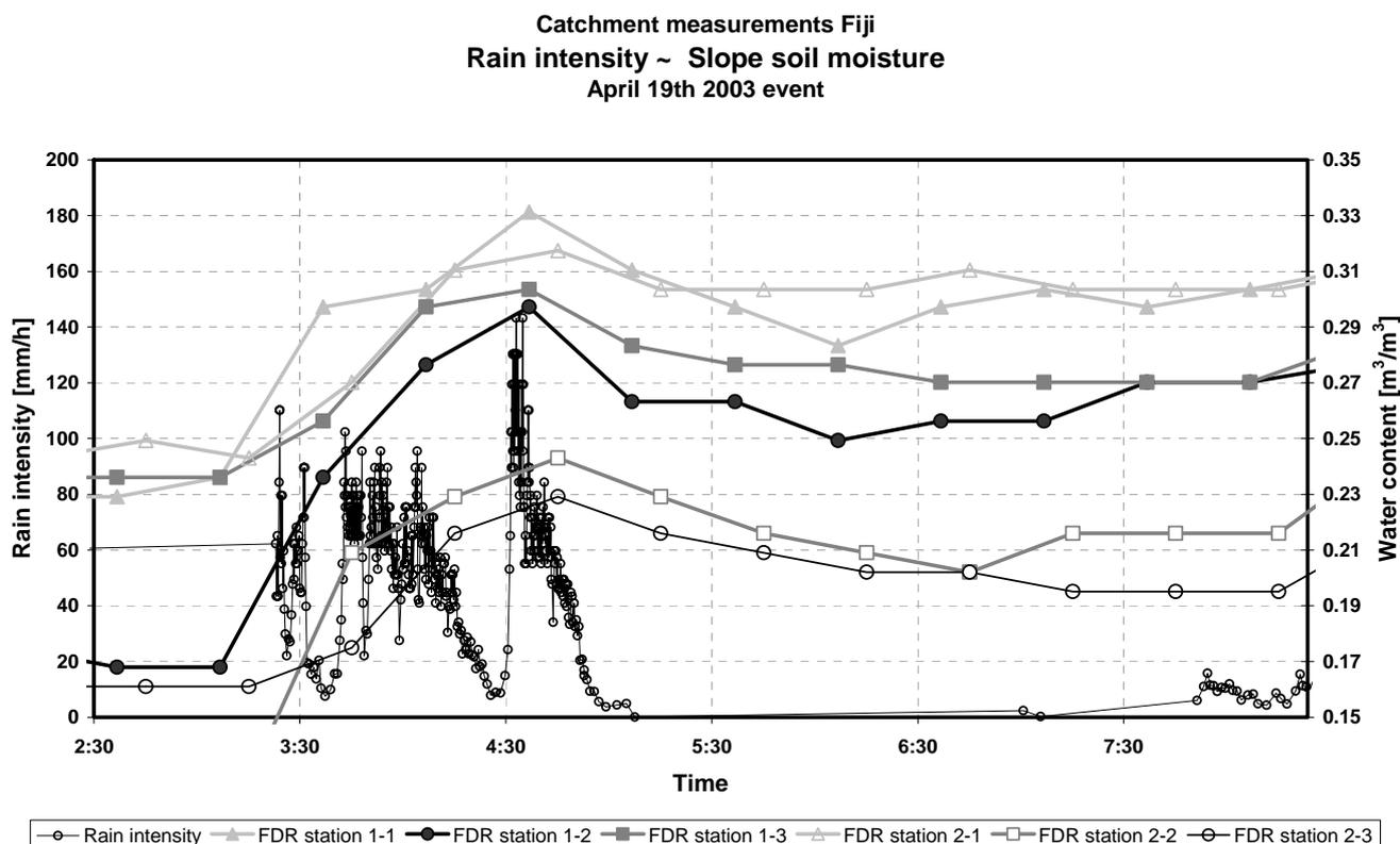
**Figure 2. Rain intensity and soil water content on two positions on a slope, each measured at three depths, in time. The solid bullets are measured by the upper FDR station, the open bullets represent the lower FDR station. The sensors were installed at -5, -10 and -20 cm.**
