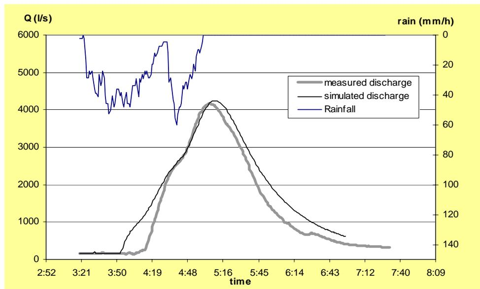
**Figure 3. Measured and calculated discharge for an event on 19<sup>th</sup> April, 2003 for the Savutalele catchment, Fiji.**
