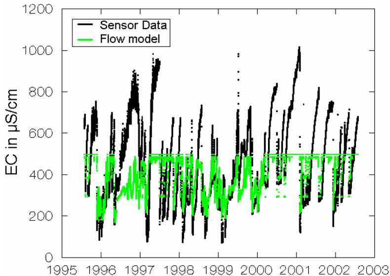
**Figure 2. EC Sensor data compared with instantaneous flow model over time. No flows are a constant.**
