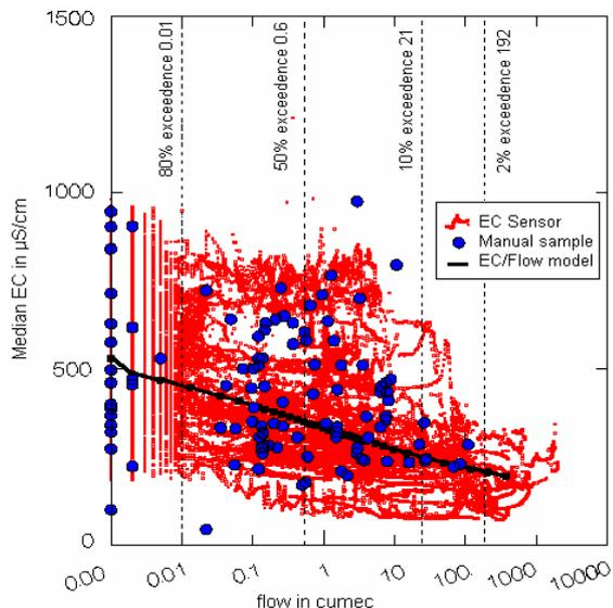
**Figure 1. Flow/EC relationship modelled for instantaneous flow on Condamine River**
