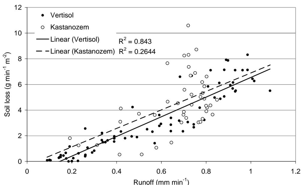
**Figure 2. Runoff-soil loss relationship illustrating lower variability of erodibility on the Vertisol than the Kastanozem**
