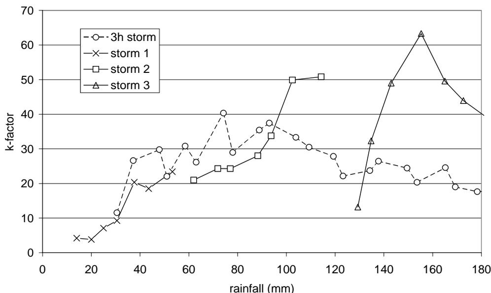
**Figure 1. Kastanozem interrill erodibility during three-hour and three one-hour storms**
