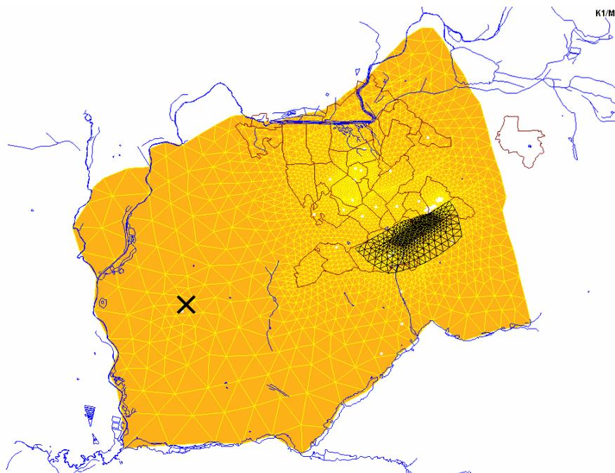
**Figure 3. Model mesh, placement in the river network, and sub-model used for calibration of dual-porosity properties [black]. Position of the leaching fields (contamination) [brown] and position of the well [cross].**
