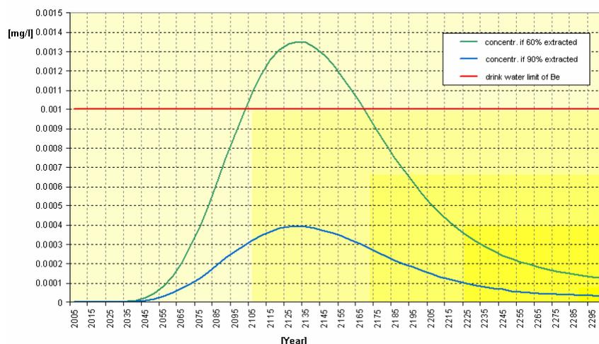
**Figure 4. Run of the concentration of contaminant (beryllium) in the drink water well for two scenarios with different ratio of decontamination (percent of total initial mass).**
