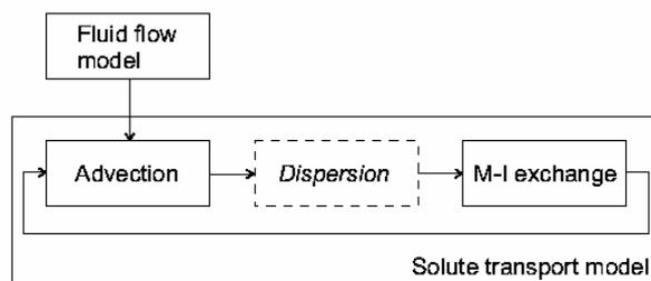
**Figure 1. Block scheme of the operator-splitting approach for solution of the non-equilibrium dual-porosity transport.**
