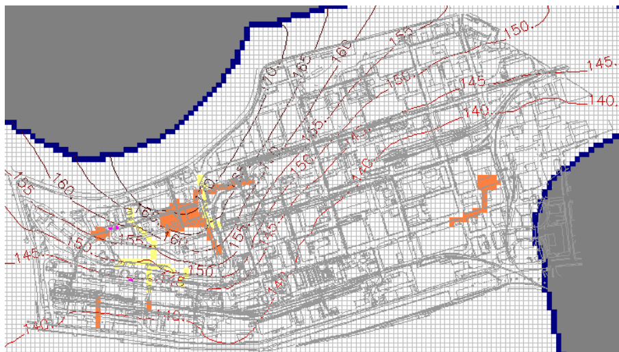
Figure 1. Scheme of the chemical factory with part of the model mesh and isolines of piezometric head.
