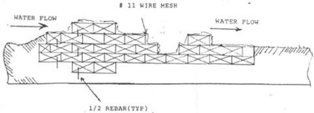
SIDE VIEW OF TYPICAL TIRE DAM MADE OF 5.5 X 4.5 X 2.5 TIRE BALES
